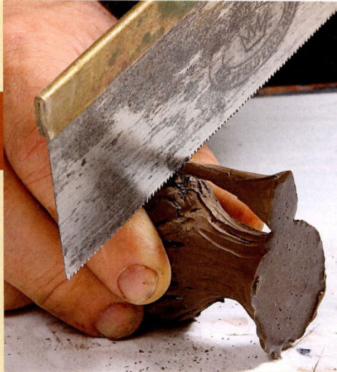
Trim the casting. The urethane resin can be worked like wood. Grove sawed off the vent, trimmed off the paper-thin flashing at the seams, sawed off some of the base, and then flattened it on a disk sander.
