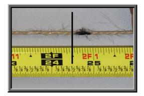
For the inside diameter (ID), stick a piece of masking tape around the inside of the collar until it meets itself, pull it off, measure it, and divide by 3.14. It is a nightmare when the ductwork (spiral pipe, fittings and flexible hose) arrives and the installer cannot make the initial connection.
