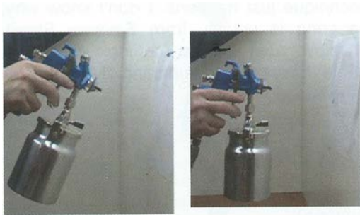
Tipping the gun results in more finish at the bottom of the pattern than at the top.
