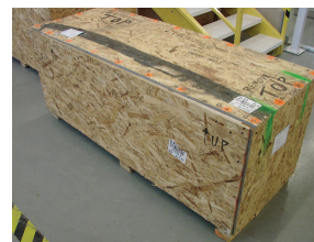
4 x 4s allow space for a forklift under this crate.
